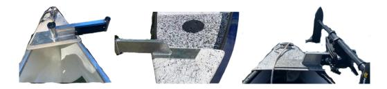
\*Warning\* always check trolling motor bracket clamp screws for tightness / damage prior to trailering, after trailing, and use on water to prevent bracket from loosening and falling off of the aluminum mount. Remember, the only thing holding the trolling motor onto the trolling motor mount is pressure from the clamp screws. Removing the trolling motor during trailering is recommended. LRC is not responsible for lost or damaged trolling motors.
